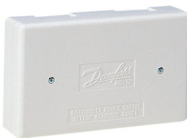
The Danfoss 12-way WB12 Wiring Centre designed for most popular heating/hot water systems. It provides a systemised and tidy approach to wiring, with cable clamps and terminal numbers. It is designed to be wall mounted, with cable entry from either the rear or through knock-outs in the rear. The following wiring connection information covers most popular domestic heating control systems.
