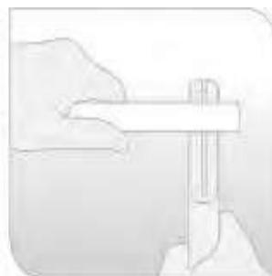
Use only purpose designed pipe cutters and cut the pipe squarely. Ensure the pipe is free from burrs and scratches.
